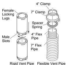
Figure 11 - Vent Pipe Connections
